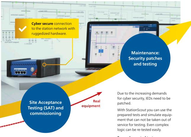
On-site tests have to be performed at least once with real equipment. Testing every point within the SCADA system (including all details) can be performed by simulating the client even without a control center.
