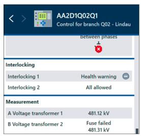
The IED summary uses clearly understandable and editable names instead of IEC 61850 abbreviations. Information is grouped according to their application, which helps the engineer trace signals. Easy to use browsing and navigation
